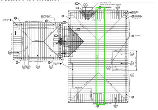
A35: An interior bearing wall is not necessary. The trusses as shown can be constructed.
